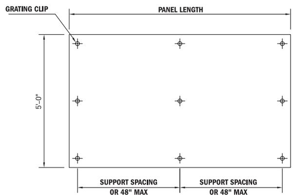
Provide a minimum of 1½" bearing surface per support.
