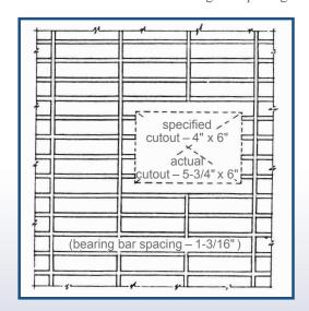
Cutouts for circular obstructions are recommended to be at least 2" larger in diameter than the obstruction. It is further recommended that cutouts for all piping 4" or less be made in the field.
