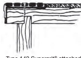
Type 142 Supergrit® attached to wood tread and backed with tile, carpet, or other material.
